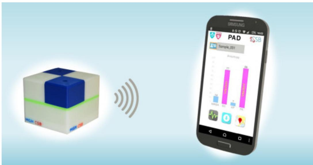
**Caption:** PAD system. Left, four optical testing cubes (blue and white) stacked on the electronic base station (white with initials); right, a smartphone with a special app to receive test results transmitted by the electronic base station.
